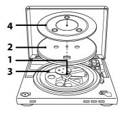
1 Move the metallic parts inside the larger gear in the direction of the arrow.
